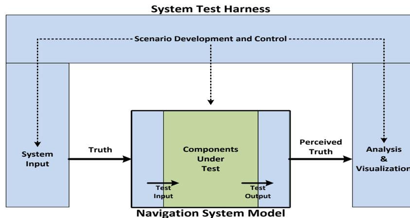
Figure 1. Framework Conceptual Configuration.
