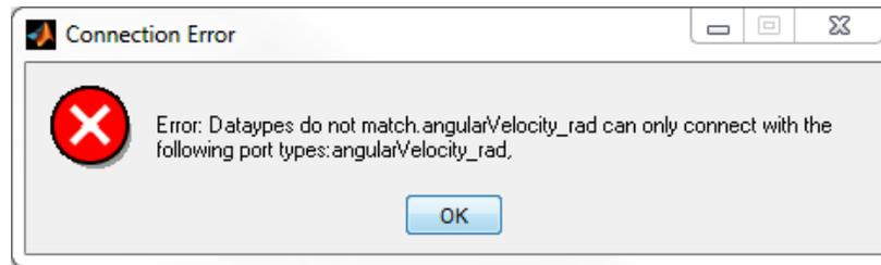
Figure 5. Sample Simulation Error Message.
